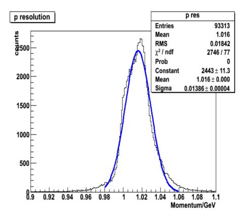
$$\left(\frac{\sigma_{pt}}{p_t}\right)_{pos} = \frac{3.3 \times 10^2 \times \sigma_x}{B \times L^2} \times p_t \times \sqrt{\frac{720}{n+5}}$$
